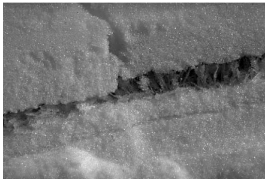
Figure 8.9: A typical weak layer composed by hoar crystals buried under a cohesive snow slab (from Jamieson and Schweizer [315]). Note the collapsed crystal structure and the detachment of the upper layer.
