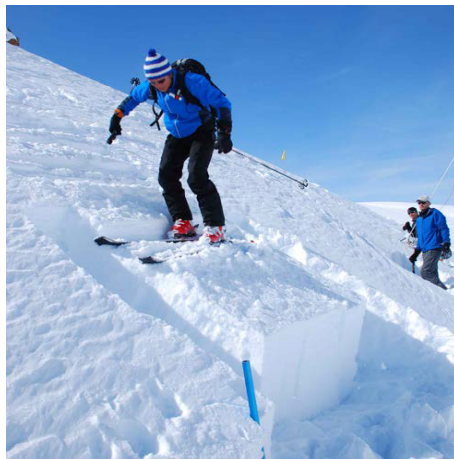
(c) Rutsch-block test
