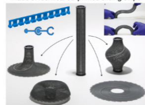
Example of morphable tubular meta-surface made of identical 3D printed sliding strips
