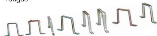
Subdomain deformation modes of an omega pultruded beam obtained with the ROM
