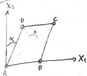
2D solid contained in  $\{x_1, x_2\}$  plane relative to an orthonormal cartesian basis  $\{e_i\}$   $i=1,2,3$ . The solid is initially square and is enclosed in a rigid truss frame hinged at the corners A, B, C and D so that the sides cannot change their length. The deformation is presumed homogeneous and is parametrized by the angle  $\alpha$ .
