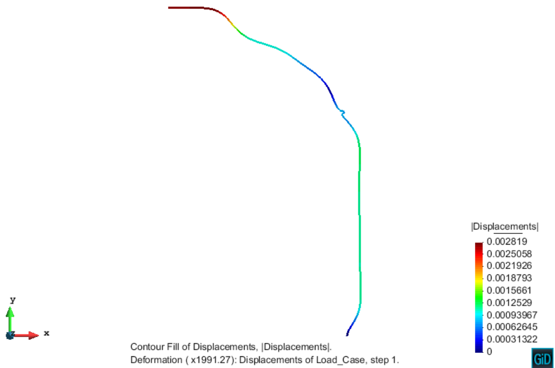
Figure 1.12: Deformed shape of the tank.
