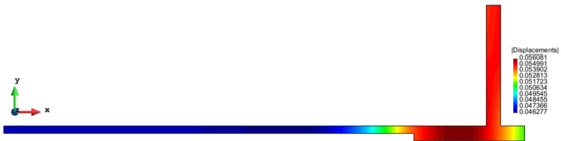
Figure 3: Total displacements [mm]
