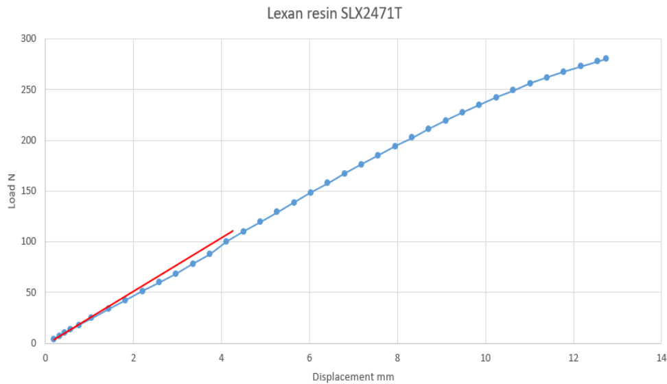
Fig 10: Load-displacement graph for SLX2471T.
