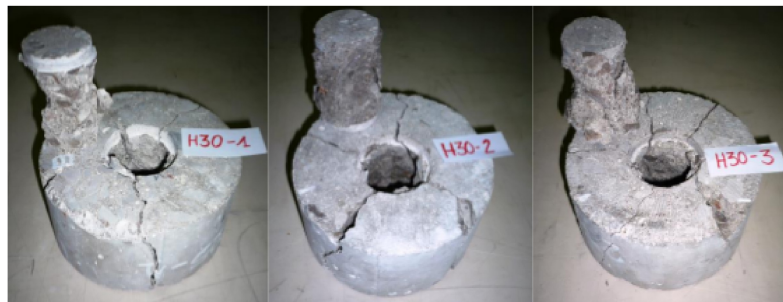
Figure 57: Fracture of H30 sample in a shear test
