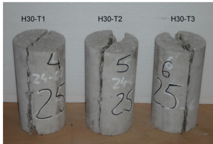
Figure 35: Fracture of the samples at Lab with concrete H30
