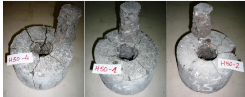
Figure 58: Fracture of H50 sample in a shear test
