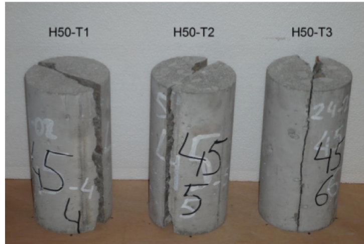
Figure 36: Fracture of the samples at Lab with concrete H50
