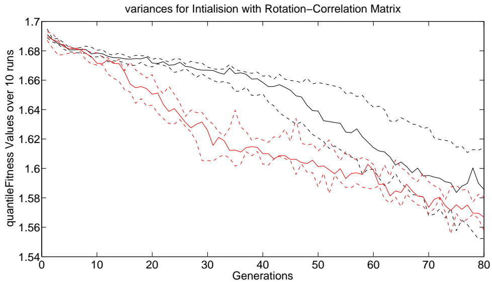
Figure 6.12: Comparison of the variance in fitness values of the full rank covariance matrix initialised with rotation-correlation matrix. Compared initialisation using correlation with rotation (red) with standard initialisation (black): lower and upper dotted lines indicate 25% and 75% of the fitness values respectively. Solid line represents the median values.
