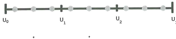
Figure 3.5: Gauss points inside each knot span.
